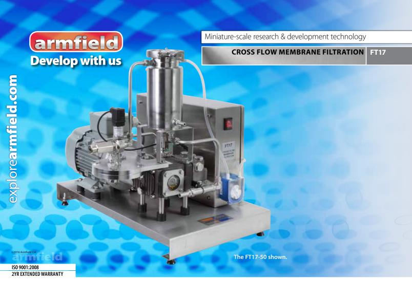
The Armfield FT17 is a lab-scale system for evaluating membranes in a cross flow filtration application enabling rapid determination of cross flow filtration performance using a range of membrane types with small product volumes (1 litre). It can also be used in teaching applications to demonstrate features of different membrane types and the effect of varying filtration variables.
