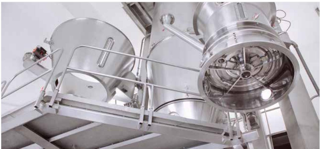
The ProCell series combines the innovative spouted-bed concept with the flexibility and multi-zone concept of a GFG. The main areas of application are the granulation of fine particles, processing of materials that are sensitive to temperature and retention time, and processing of sticky materials.
