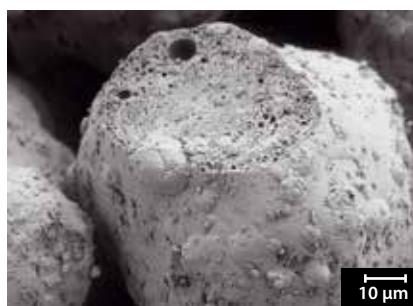
Granule with oil encapsulated in the matrix
