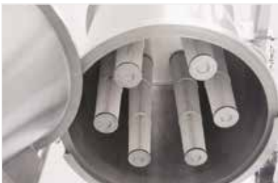
cartridge filter, internal process filter
