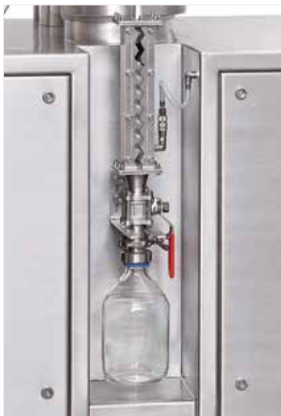
continuous product discharge/zig-zag-sifter
