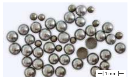
hollow spheres, powder layering, shovel rotor
