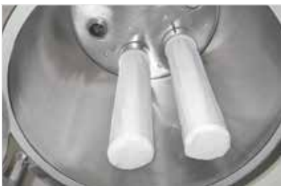
bag filter, internal process filter
