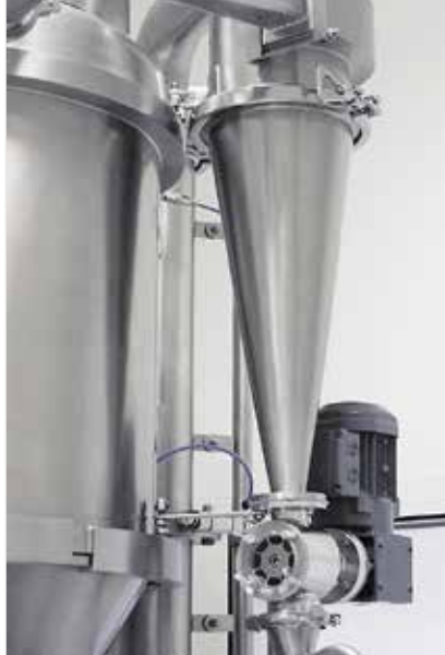
cyclone with rotary valve and dust recycling
