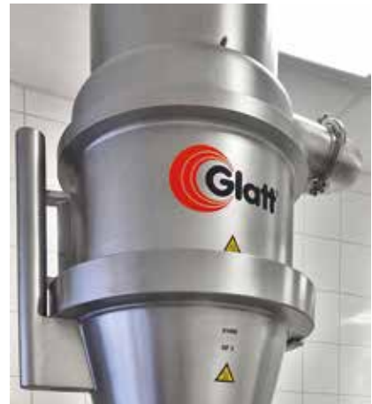
expansion chamber and filter housing in PRO-design
