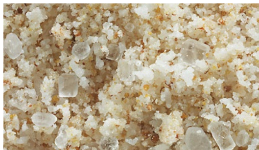
Fig. 6: Spray agglomeration improves the properties of ingredients for instant drinks; dust-free particles with a porous structure are easy to dose, wet and dissolve. Hereby particle size of raw materials has an important influence on the final product homogeneity.
