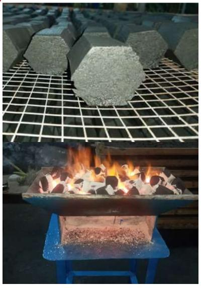
Coconut charcoal is a product made from coconut shells, which are carbonized and then activated. The product is black in color and comes in various forms based on the shape such as Barbecue Charcoal and briquettes. In recent years, the demand for
