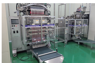
Filling and Packaging Facility-stick filler
